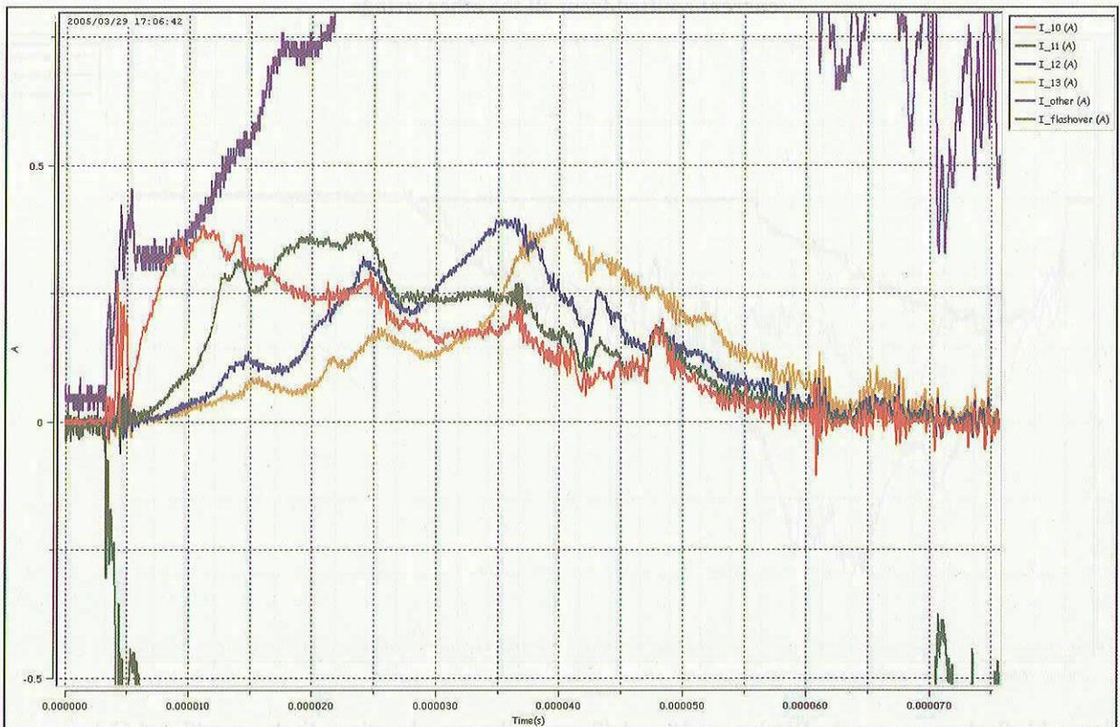
Figure 15: current emitted by strings n°10-13 during discharge 47. Plasma propagation speed was calculated using peak currents and give value from  $0.7$  to  $1.1 \cdot 10^{+4} \text{ m.s}^{-1}$ .
