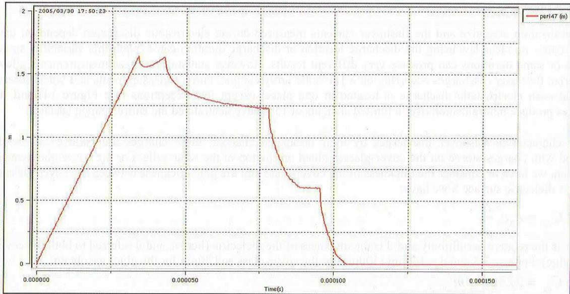
**Figure 16: perimeter calculation.** From the same location than the discharge 47, and using  $0.77 \cdot 10^4$  m/s as the propagation speed, we calculated the perimeter evolution with time of a plasma bubble created at the discharge location.
