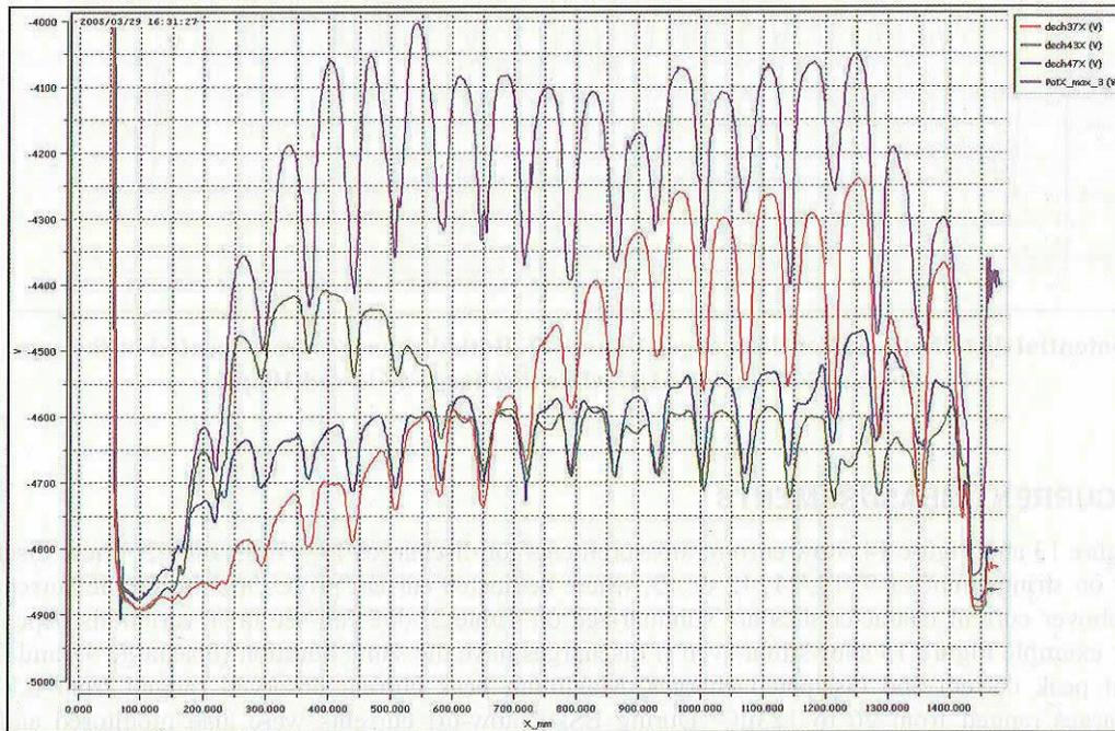
Figure 9: potential distribution on the X-axis after discharges 37, 43 and 47.
