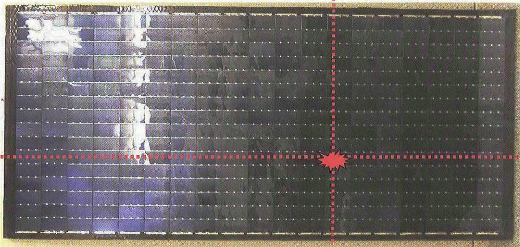
**Figure 3: Sample made of 19\*16 solar cells (silicon). The red cross represent the way the potential distribution was measured around the discharge location.**
