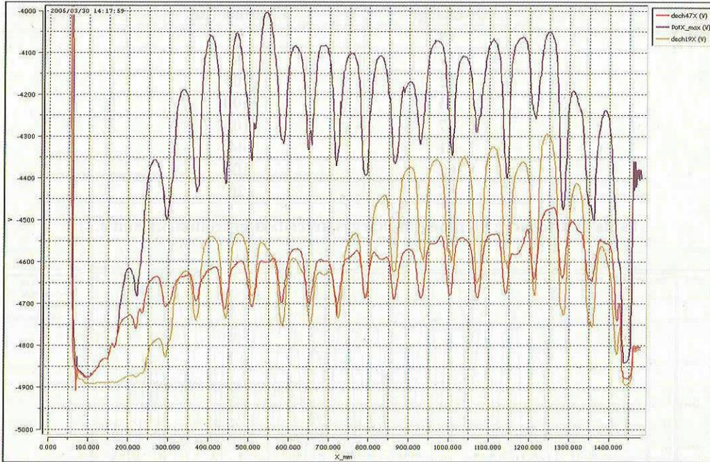
**Figure 11: potential distribution after discharges 19 and 47. Both discharges were located in the same place, but discharge 19 lasted 51 $\mu$ s while discharge 47 lasted 106 $\mu$ s.**
