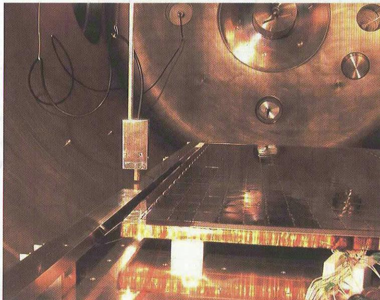
**Figure 4: sample, vacuum chamber and surface potential probe.**
