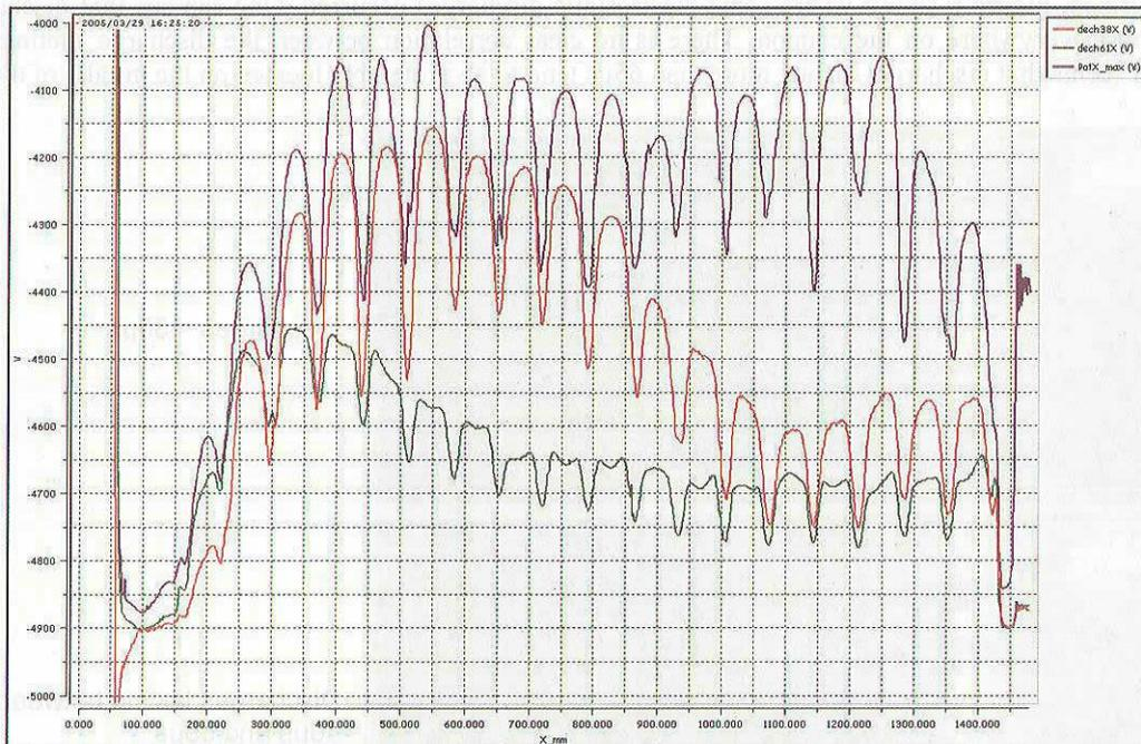
**Figure 7: surface potential distribution on the X-axis. PotX\_max shows the maximum differential voltage obtained after 12mn of irradiation. Dech38X and dech61X show the potential distribution after respectively discharge n°38 and 61.**
