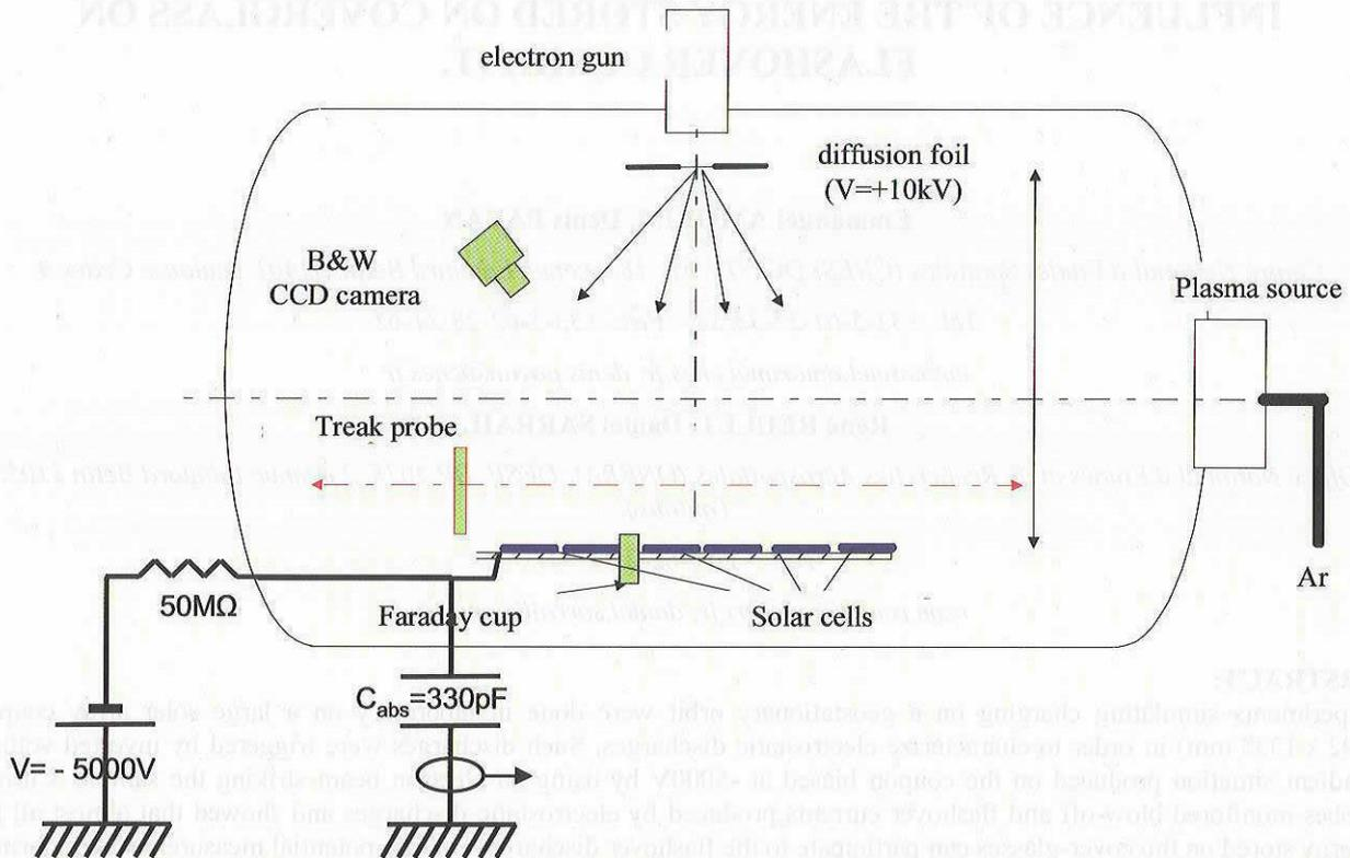
**Figure 1: Experimental set-up: schematic view. The sample is put in vacuum and biased to -5kV and irradiated by an electron beam. Probes monitor currents during ESD and a non-contacting potential probe performed surface potential distribution. The plasma source was used after each discharge to reset the differential voltage.**
