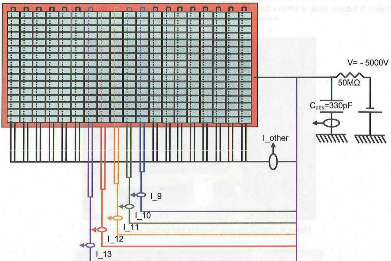
**Figure 2: Current measurements schematic view: current passing through strings 9 to 13 are monitored using current probes. Both wires of each string are connected together and measured by the same current probe. Wires of all the other strings are also connected the same way and measured by another current probe (I<sub>other</sub>). The blow-off current was also measured by monitoring the 330pf capacitor discharge.**
