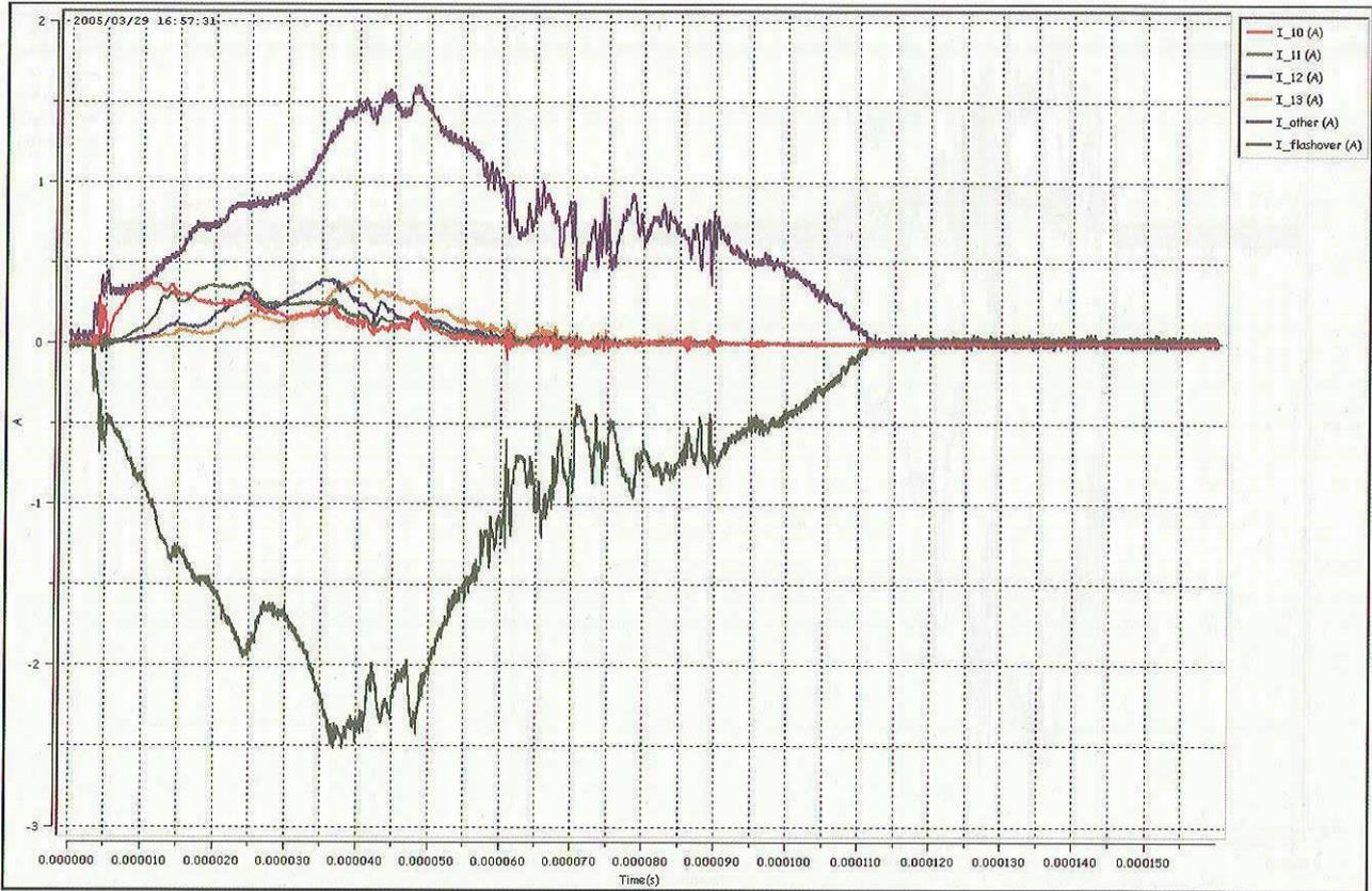
Figure 12: Current measurements obtained on discharge 47. The discharge was located on string n°9: I\_9 gives the flashover current while I\_10 to I\_13 give the current emitted from the strings n°10-13. I\_other shows the current emitted from all the other strings.
