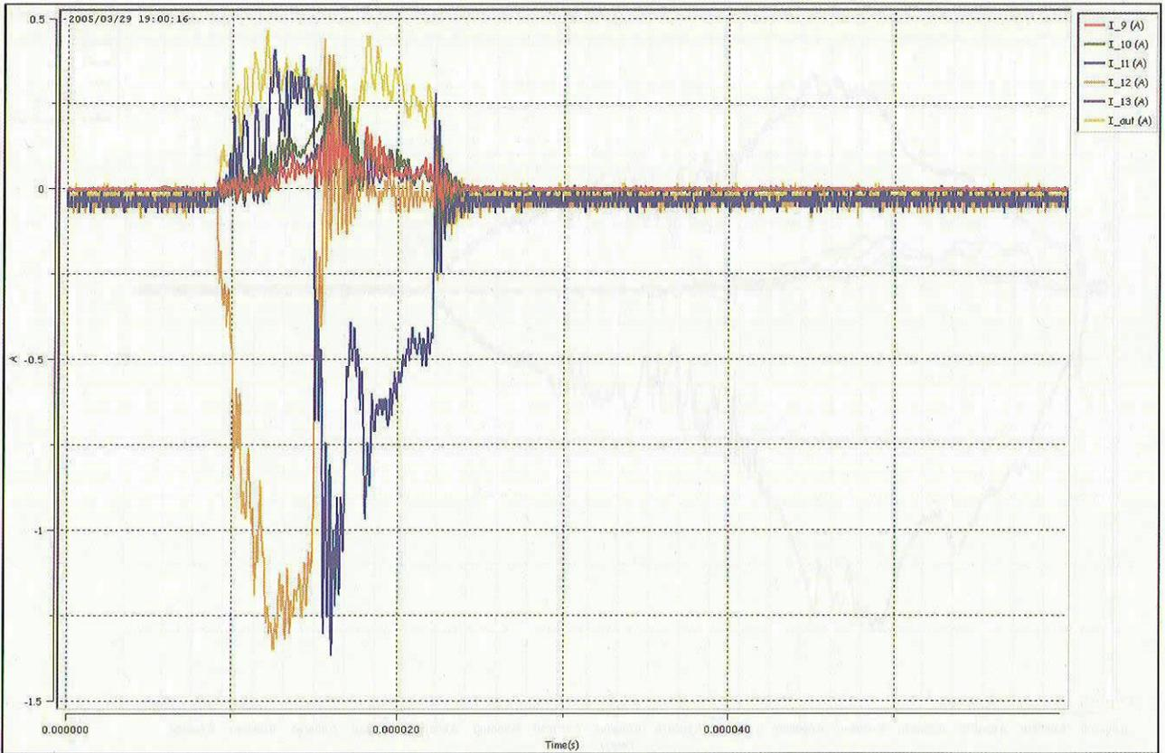
Figure 14: discharge 53: the only case of flashover current seen on different strings. Here the flashover current is received first by string 12, then by string 11 showing the discharge location has moved.
