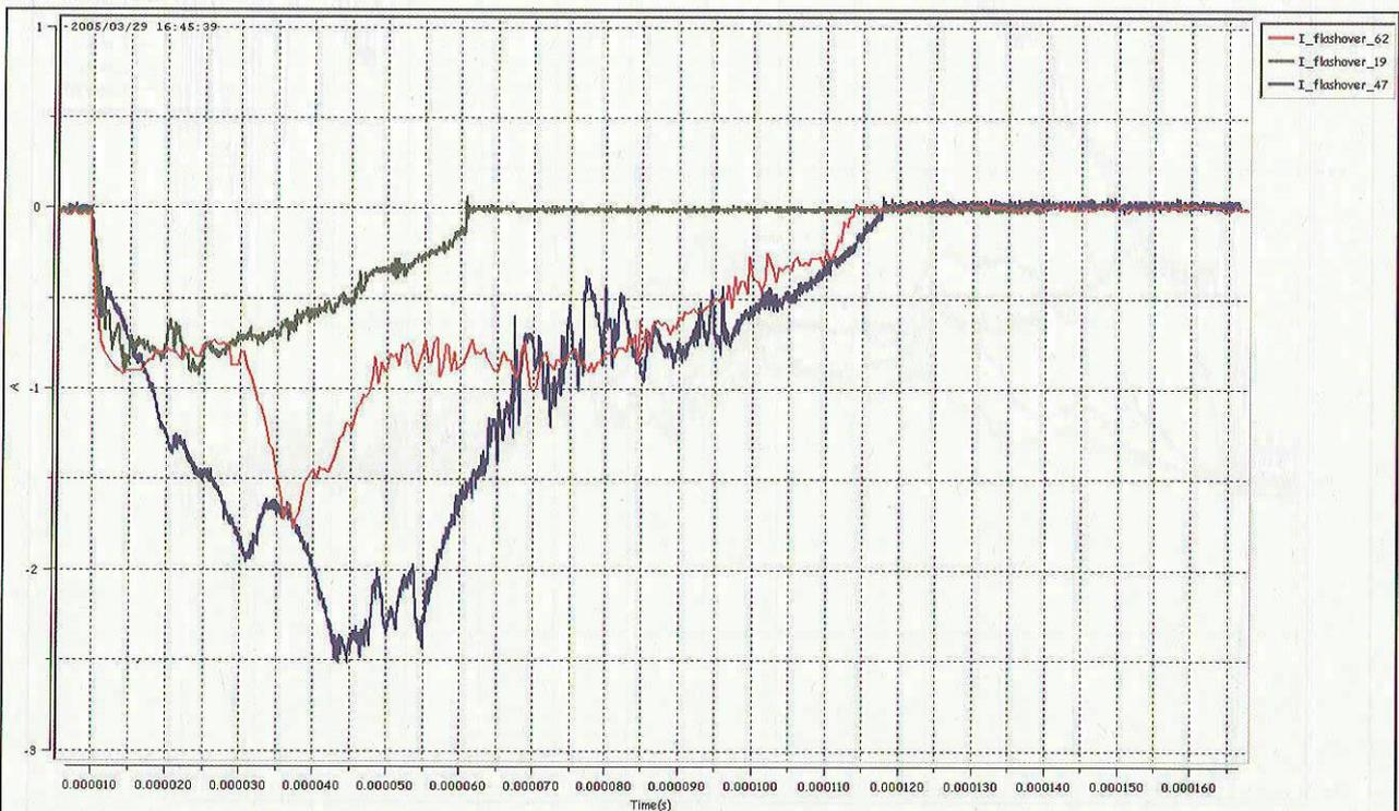
Figure 13: flashover currents. Discharges 19 and 47 are on the same location, discharges 47 and 62 have same duration but peak current and dissipated charges are different.
