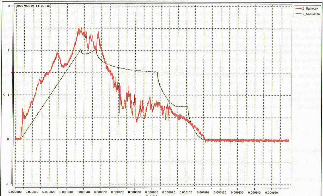
**Figure 17: flashover current measured during discharge n°47 and current calculated based on plasma calculation.** Current waveform doesn't fit exactly the experimental curve but dissipated charges are the same:  $125 \mu\text{C}$ .
