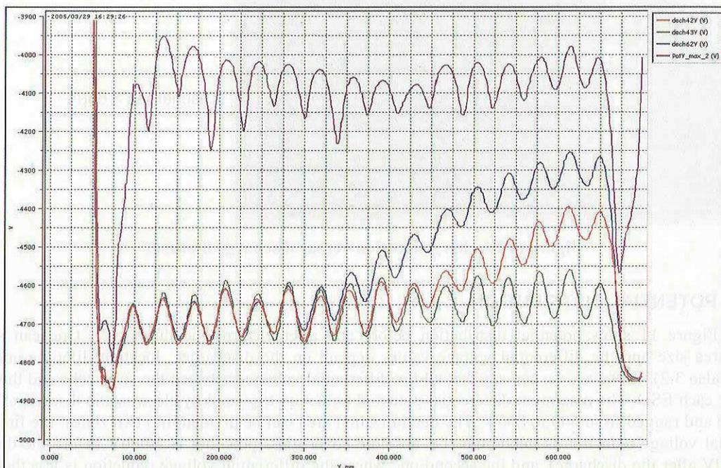
**Figure 8: potential distribution on the Y-axis after discharges 42, 43 and 62. PotY\_max shows the maximum differential voltage obtained after 12mn of irradiation.**
