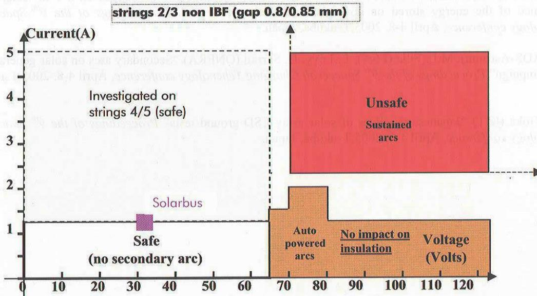
The Solarbus solar array design offers a security margin of 2 versus the arc voltage threshold (33 V versus 65 V).
