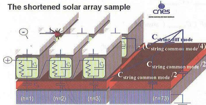
**Figure 8** : The shortened solar array sample and the missing capacitances
