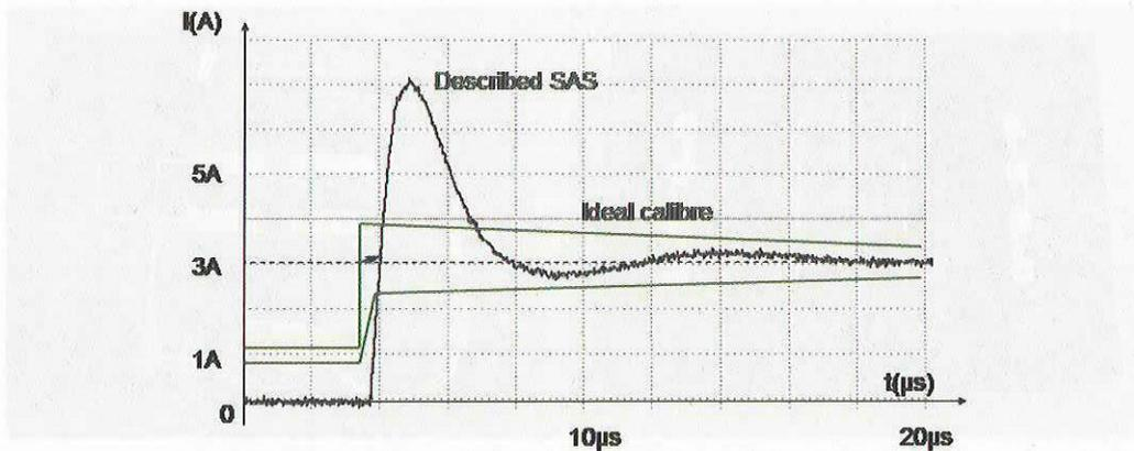
**Figure 4** : Example of a measured power source switch response
