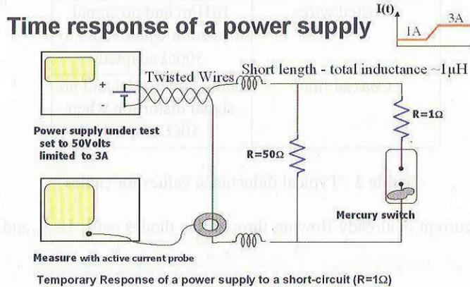
**Figure 3** : Schematic diagram of power supply test circuit
