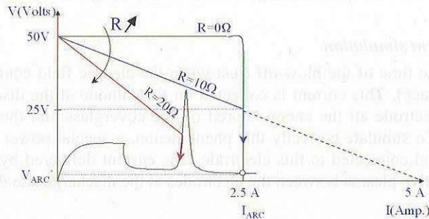
**Figure 10** : Effect of an added resistance in the discharging circuit (SAS + resistance)
