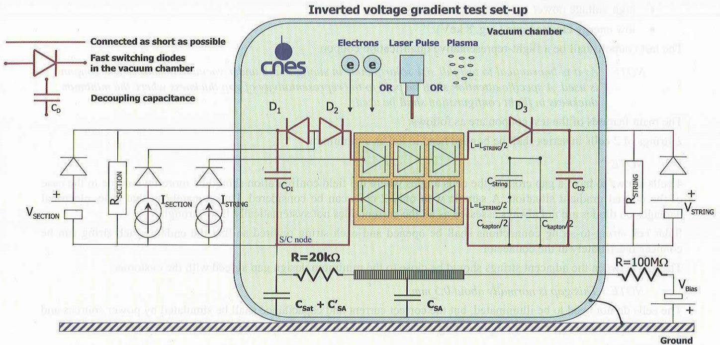
Figure 1 : Solar array test set-up
