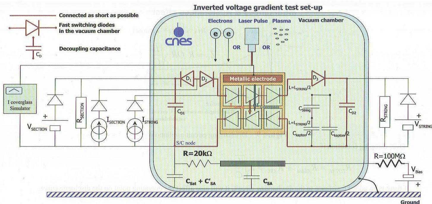
Figure 11 : Setup simulating the satellite including flashover current
