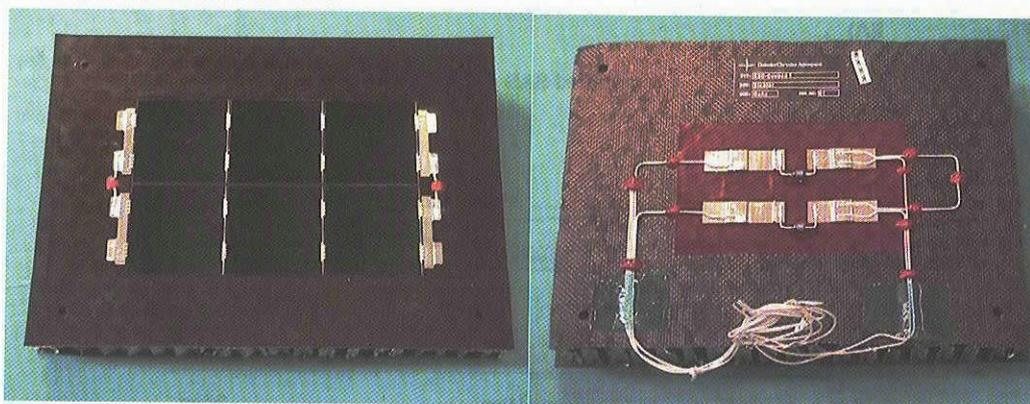
**Figure 2** : Photograph of solar cells sample – Front face & Rear face (Stentor Sample. Picture from Denis PAYAN-CNES®).
