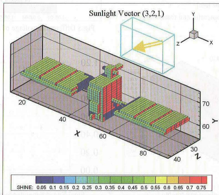
Fig.8 Ray tracing model of OICETS (100x128x64 grids)
