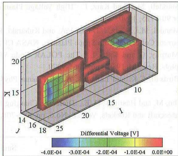
Fig.5 Differential voltage of a satellite model
