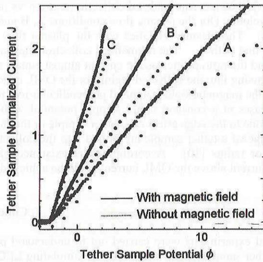
Fig.8 Normalized collection current vs normalized tether sample potential characteristics varying plasma velocity (for plasma flow conditions A, B and C) at tether sample diameter and length of 0.4 and 52 mm, respectively, with magnetic field.
