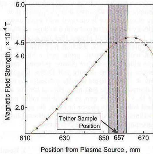
Fig.1 Ground experimental system of spacecraft bare tether. Fig.2 Axial distribution of magnetic field strength on central axis of plasma source. The magnetic field strength was measured with a Hall sensor.
