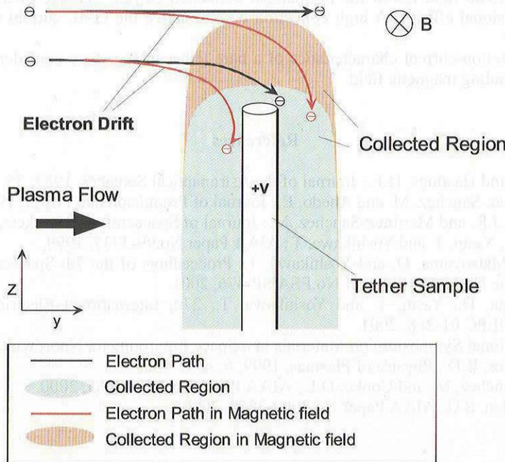
Fig.9 Feature of electron collection for bare tether with magnetic field.
