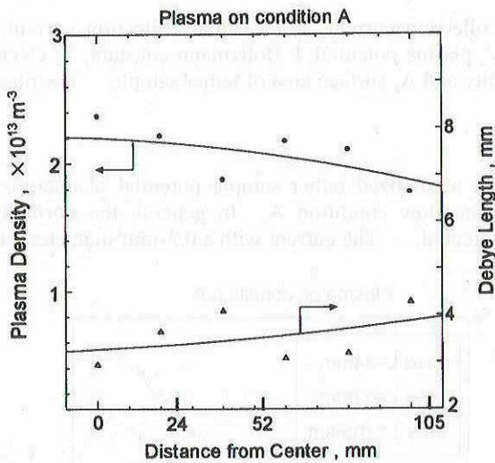
Fig.3 Radial distributions of plasma number density and Debye length at plasma flow condition A without magnetic field.
