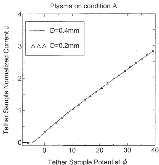
Fig.5 Normalized collection current vs normalized tether sample potential characteristics varying tether sample diameter at constant tether sample length of 52 mm for plasma flow condition A without magnetic field.
