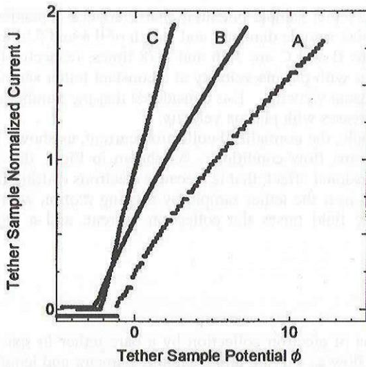
Fig.7 Normalized collection current vs normalized tether sample potential characteristics varying plasma velocity (for plasma flow conditions A, B and C) at tether sample diameter and length of 0.4 and 52 mm, respectively, without magnetic field.
