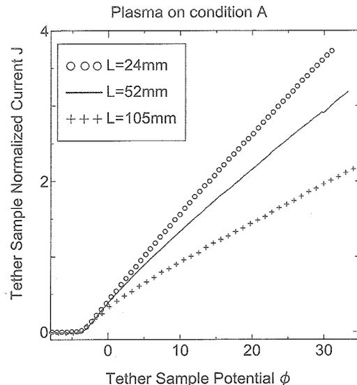
Fig.6 Normalized collection current vs normalized tether sample potential characteristics varying tether sample length at constant tether sample diameter of 0.4 mm for plasma flow condition A without magnetic field.
