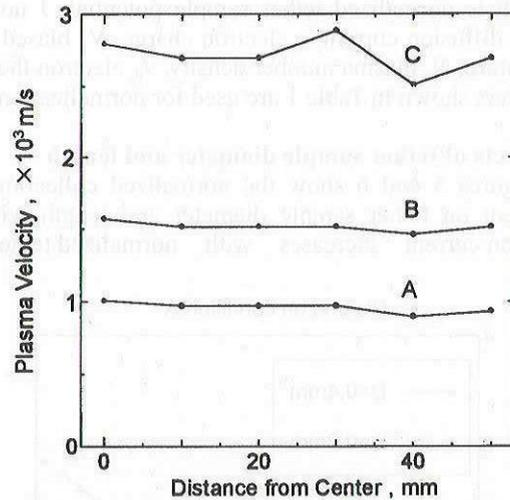
Fig.4 Radial distributions of axial plasma velocity at plasma flow conditions A, B and C without magnetic field.
