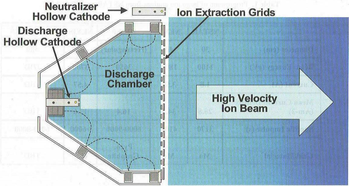
Figure 2. Basic operation of an ion engine. Note that the “Ion Extraction Grids,” which consist of the screen and accel grids, and which are shown here as flat, are usually dished for space operation.
