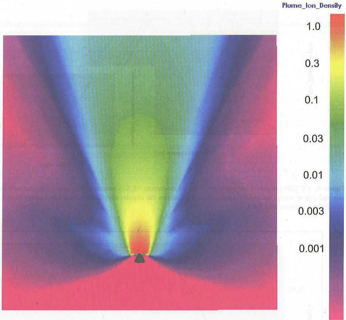
**Figure 6.** Two-dimensional representation of NEXIS plume, calculated by PlumeTool and displayed in EPIC. Note presence of charge-exchange ion plume extending well beyond 90 degrees from thruster axis.
