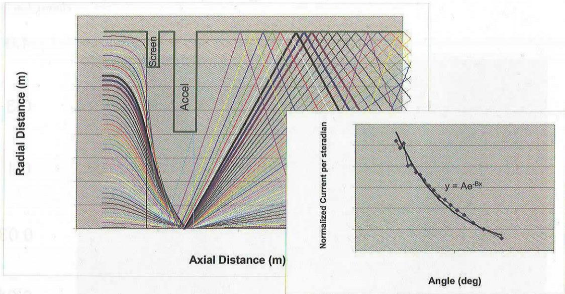
**Figure 4.** CEX2D-calculated ion trajectories for a low-current NEXIS beamlet. Numerous trajectories bounce off the axis and exit at angles up to 30 degrees. The inset shows the angular distribution for a low-current beamlet, which is well-fit by an exponential form.
