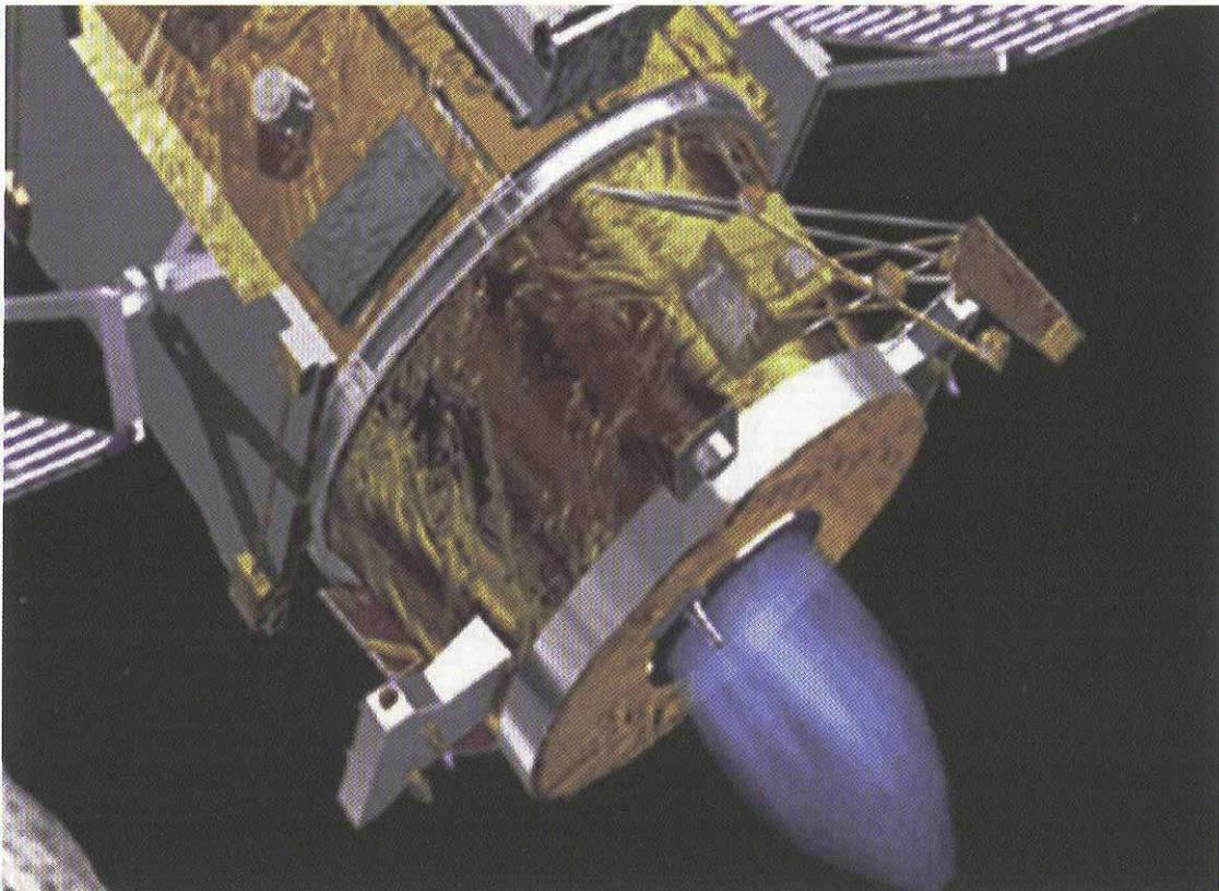
**Figure 1.** The NSTAR thruster completed a mission of over 16,000 hours as part of the DS1 spacecraft.
