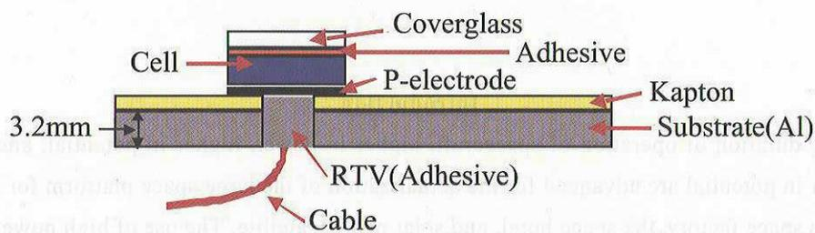
Fig.2 Structure of Solar Array Coupon
