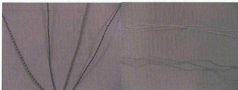
Fig. 17 Braiding type tether (left) and net type tether (right)
