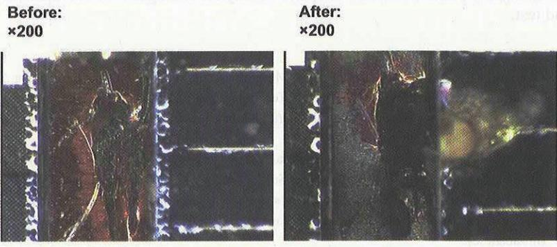
Figure 28: Damages due to Arcs
