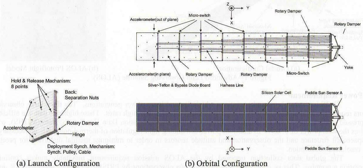
Figure 3: ALOS Solar Array Paddle
