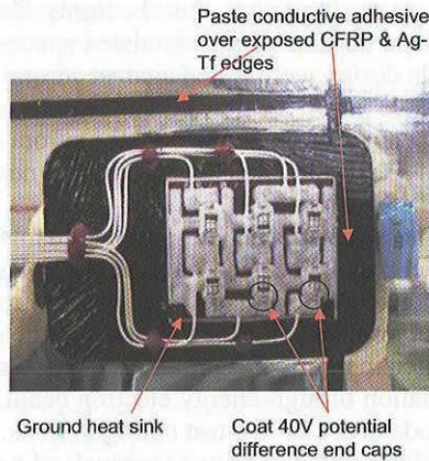
Figure 16: Bypass Diode Board Modifications
