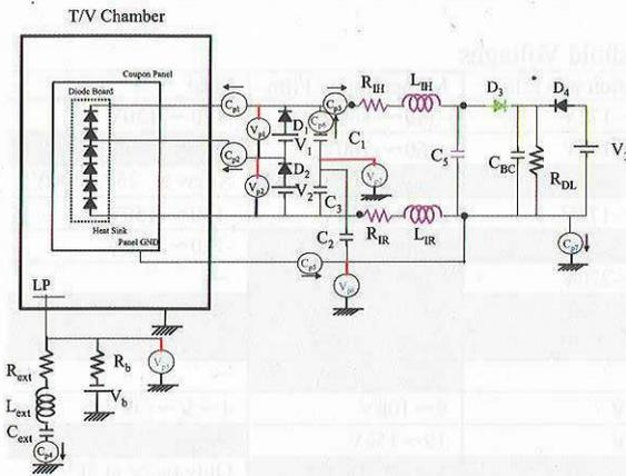
(c) Electron Beam Test (Shunt off)
