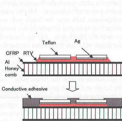
Figure 15: Conductive Adhesive Coating
