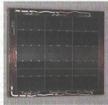
Figure 26: Panel Frontside Coupon
