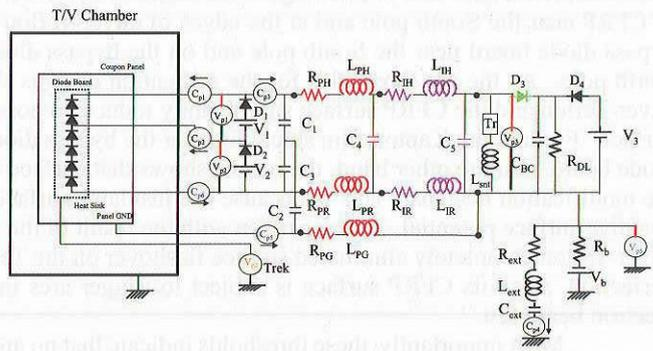
(b) Plasma Interaction Test (Shunt on)
