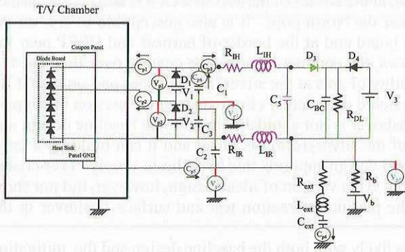
(a) Plasma Interaction Test (Shunt off)
