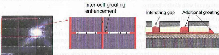
Figure 17: Grouting Enhancement
