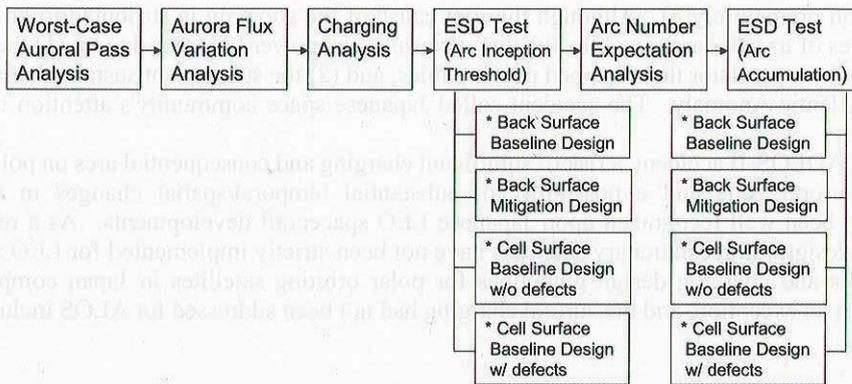
Figure 8: Charging Analyses and Verification Process
