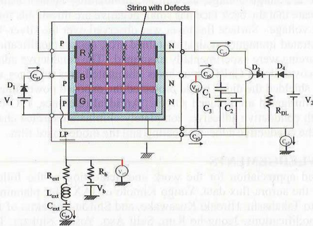
Figure 25: Electrical Block Diagram of Panel Frontside ESD Tests
