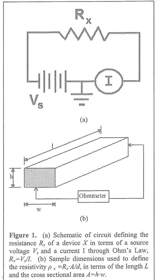
Figure 1. (a) Schematic of circuit defining the resistance  $R_x$  of a device  $X$  in terms of a source voltage  $V_s$  and a current  $I$  through Ohm's Law,  $R_x = V_s/I$ . (b) Sample dimensions used to define the resistivity  $\rho_x = R_x \cdot A/d$ , in terms of the length  $L$  and the cross sectional area  $A = h \cdot w$ .
