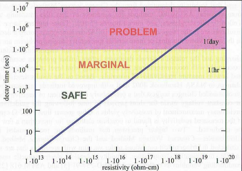
**Figure 6.** Decay time as a function of resistivity based on a simple capacitor model and Equation (1). Here  $\epsilon_r$  is set to 1. Marginal charging problems occur for materials with resistivities (or more properly  $\rho \cdot \epsilon_r$ ) in excess of  $\sim 4 \cdot 10^{16}$   $\Omega\text{-cm}$ , when the decay time  $\tau$  exceeds ~1 hr. More serious charging problems occur for  $\rho \cdot \epsilon_r \geq 10^{18}$   $\Omega\text{-cm}$ , when decay times exceed ~1 day.
