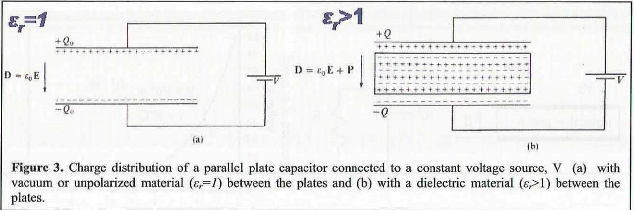
**Figure 3.** Charge distribution of a parallel plate capacitor connected to a constant voltage source,  $V$  (a) with vacuum or unpolarized material ( $\epsilon_r=1$ ) between the plates and (b) with a dielectric material ( $\epsilon_r>1$ ) between the plates.
