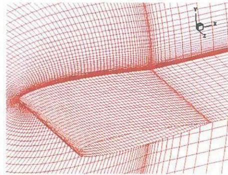
Fig.2 the grid for airfoil
