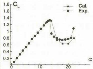
Fig.14 Lift vs. attack angle for NACA63<sub>1</sub>-012
