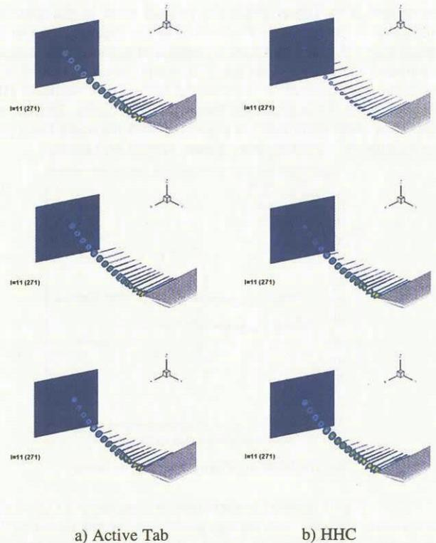
Fig. 9: Vorticity contour of tip vortex shed from blades with active tab and HHC
