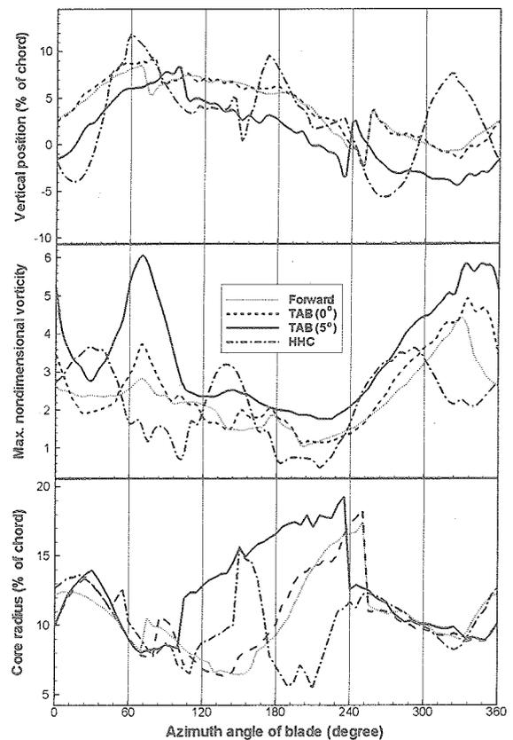
Fig. 16: Effect of tab and HHC on core radius, vorticity, and vertical position of tip vortex.
