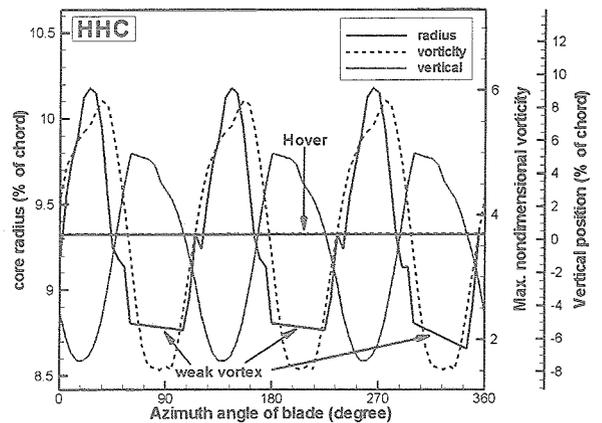
Fig. 13: Effect of HHC on tip vortex.
