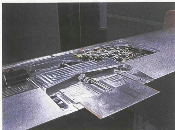
Fig.1: Active tab installed in a blade used for a wind tunnel test<sup>10</sup>
