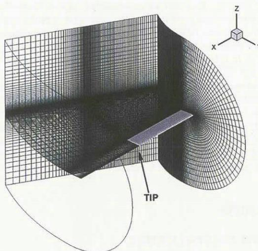
Fig.2: Grid of single blade
