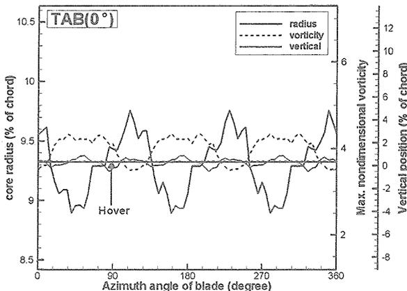
Fig. 11 Effect of Tab A on tip vortex.
