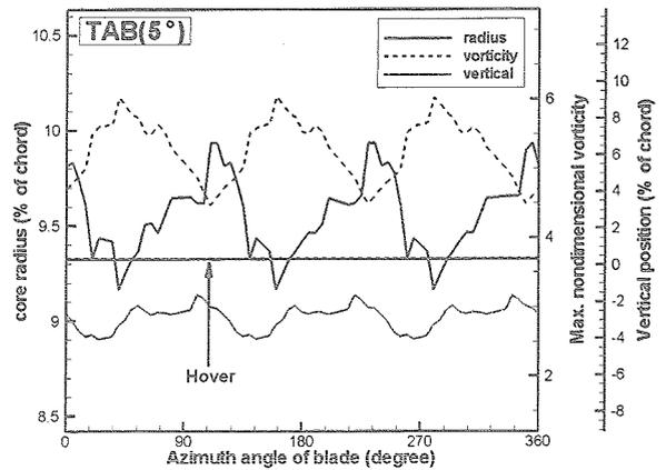
Fig. 12: Effect of Tab B on tip vortex.
