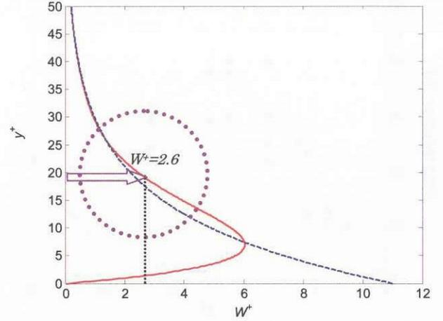
**Figure 4: Spanwise velocity profile under the Lorentz force oscillation. Solid line shows the envelope of spanwise velocity profile calculated by Berger et al. (2000); dashed line shows the calculated spanwise velocity profile when an equivalent wall velocity  $W^+_{eq}$  is introduced. (Pang et al. 2003); dotted circle shows the average location and size of near-wall streamwise vortices**
