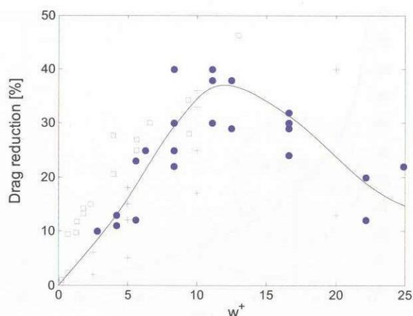
**Figure 2. Drag reduction against  $W_{\text{equi}}^+ = StT^+ / (2\pi Re_\tau)$  at all the Lorentz force oscillation conditions; Comparisons with data from Choi (2002) and Berger et al. (2000) are also shown in the figure.**
