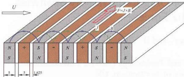
**Figure 1: Configuration of electrodes and magnets to create Lorentz force in parallel to wall surface, normal to flow direction. By switching the polarity of the electric current, spanwise-oscillating Lorentz force field was created.**
