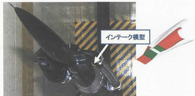
Fig. 1 Wind tunnel model for scaled supersonic experimental aircraft and intake at NAL.
