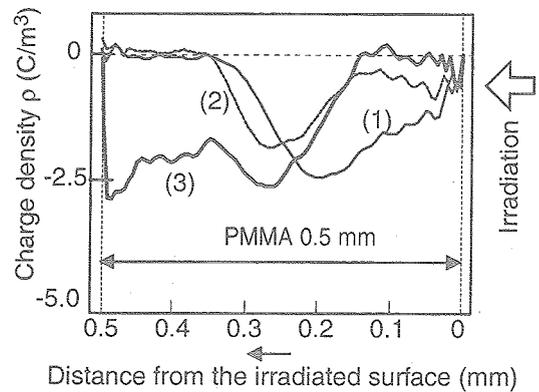
Fig. 4 Space charge profiles of a PMMA sheet under and after irradiations. (1) 200 keV, 1 nA/cm<sup>2</sup>, 4 min., (2) after 13 hrs without irradiation, (3) 300 keV, 1 nA/cm<sup>2</sup>, 4 min.
