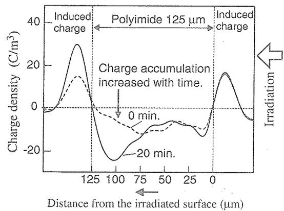
Fig. 5 Space charge profiles observed with a polyimide film under electron beam irradiation of 95 keV for 20 minutes.
