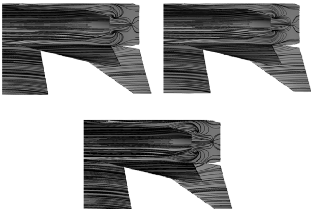
(b) NPR1.47 (左 : Mod. S-A, 右 : Mod. S-A+Anisotropic, 下, SST-k \omega )
