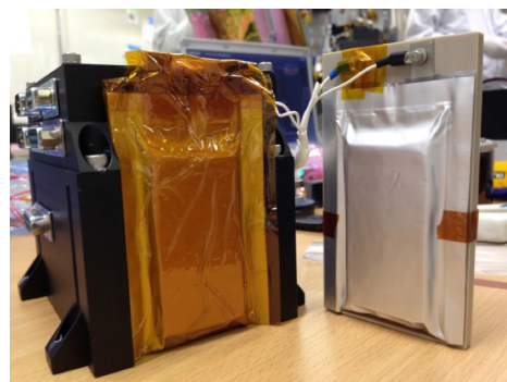
Figure 2. Photograph of the IL-LIB cells mounted on the demonstration module.
