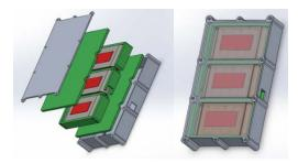
Figure 4 CAD design of battery box
