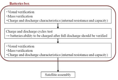
Figure 3 Battery Box assembly requirements
