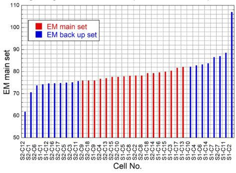
Engineeing model main and back up sets idividual cells impedance
