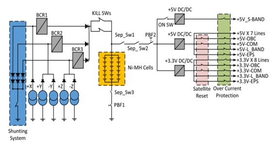
Figure 1 HORYU-IV Electrical Power Subsystem Block diagram [1]
