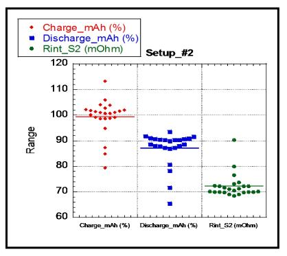
Figure 12 Range of variation of the Charged /discharged capacity and internal impedance of the cells screened by setup2
