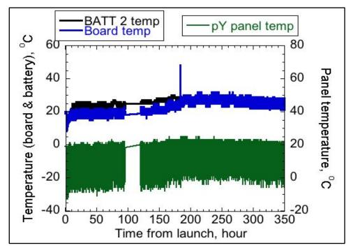
Figure 18 Battery temperatures on orbit, °C
