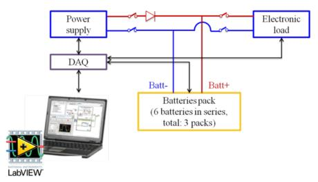
Figure 6 Block diagram of measurement setup (setup1 and setup2)
