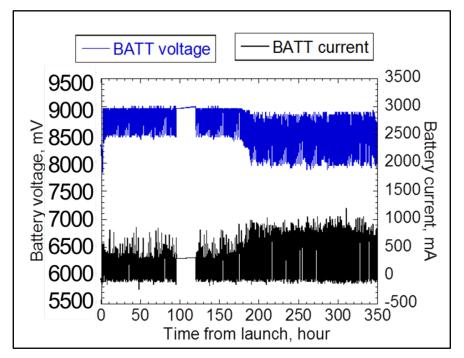
Figure 17 Battery current and voltage on orbit
