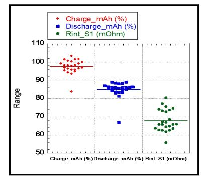
Figure 10 Range of variation of the Charged /discharged capacity and internal impedance of the cells screened by setup1
