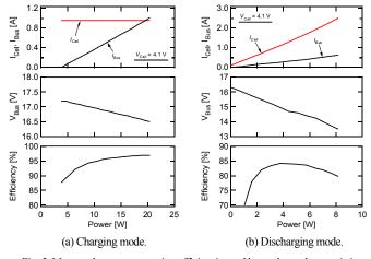
Fig. 5. Measured power conversion efficiencies and bus voltage characteristics.
