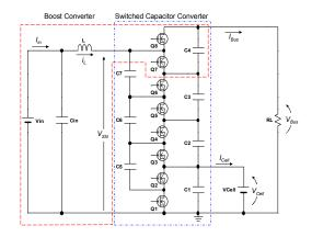
Fig. 3. 3-port converter integrating boost and switched capacitor converters.
