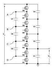
(b) Switched capacitor converter.Fig. 2. Key elements of the 3-port converter.
