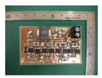
Fig. 4. A photograph of a 20-W prototype.
