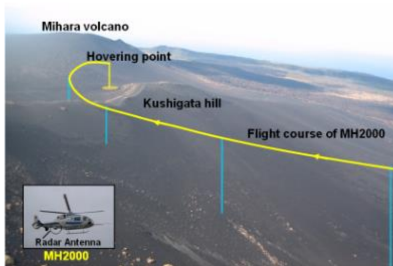
Field tests of landing radar using helicopter
