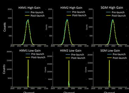
The peak channel and the width of the pedestal data for all data modes are consistent between a pre-launch and a post-launch data.
