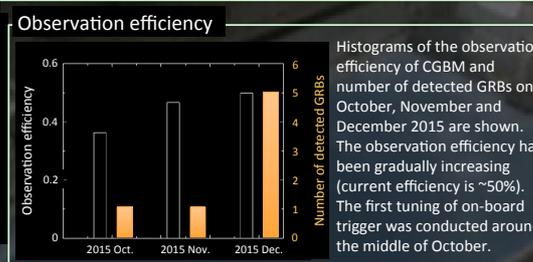
Histograms of the observation efficiency of CGBM and number of detected GRBs on October, November and December 2015 are shown. The observation efficiency has been gradually increasing (current efficiency is ~50%). The first tuning of on-board trigger was conducted around the middle of October.
