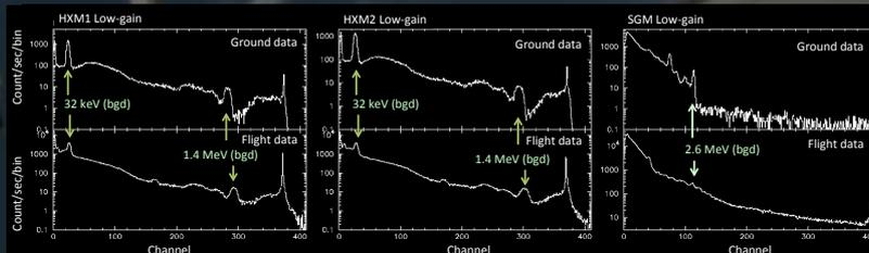
Comparison of the background spectrum between the ground data collected on March 12, 2015 and the flight data on September 22, 2015. Some internal background lines are seen in both data set. We confirmed by measuring the energy resolutions of those background lines that there is **no degradation in performance** between the ground and the flight data.
