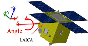
$\Delta V$  direction is designed considering: Power budget/ Thermal condition (Necessary) 2) Doppler sensitivity (If possible) Guidance direction with guidance insensitive direction as parameter.
