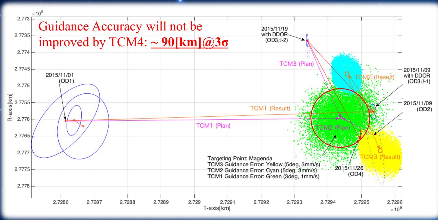
TCM 1: 0.50 [m/s] by CT-1/2 (-Z acceleration) *TCM 2*: 0.29[m/s] by CT-3/4 (+Z acceleration) TCM 3: 0.26[m/s] by CT-3/4 (+Z acceleration)
