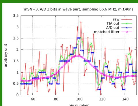
Fig 2.2 An example of the matched filtering in RFM. Red line is an input signal to RFM which is sum of the return pulse and white noise. Green line is an output from 66.6 MHz TIA. Blue line is a simulated output from 3-digit ADC. And green line is a filtered signal. SNR of the red line is 3.
