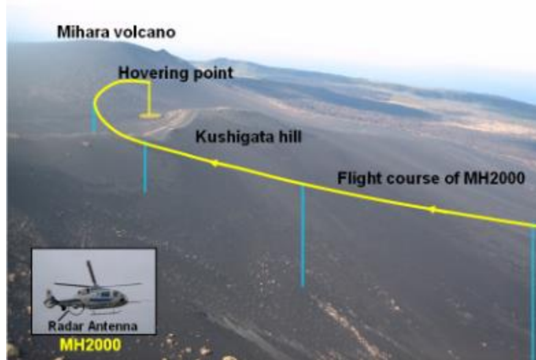
Field tests of landing radar using helicopter
